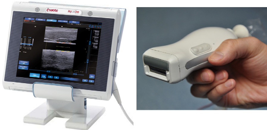
Fig. 1. Portable imaging scanner combining photoacoustics and ultrasound, left is the ultrasound scanner system, right is the picture of the probe integrating laser module and ultrasound transducer array.
