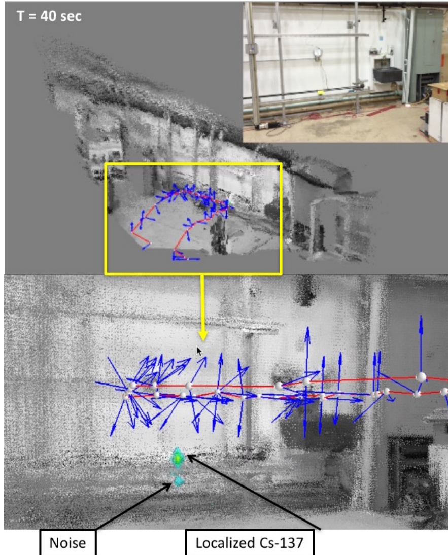
Figure 4: This shows the final reconstruction from walking around in a lab scene. The estimation for the Cs-137 source location improves as more data is collected. The blue arrows are the Compton events used in the reconstruction, the line is the path of the detector in the scene and the white circles are the location of the cone vertex.
