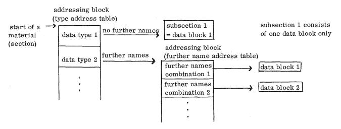
subsection 2 contains one addressing block and one or more data blocks depending on the number of combinations of further names
