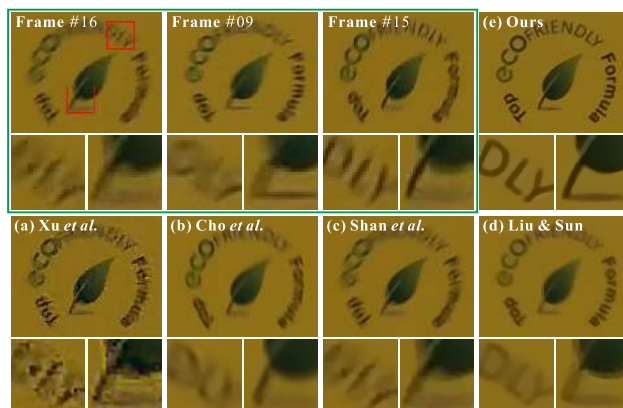
Figure 1. Multi-frame super-resolution (SR) results on a real video sequence. Green box: Input frames ( 150 \times 120 ) directly cropped from a video captured by an iPhone. Three clearest frames are shown. Motion blur and compression artifacts are present. (a) Result of single image deblurring [30]. (b) Result of video deblurring [7]. (c) Result of video upsampling [19]. (d) MFSR result [16]. (e) Our result ( \times 3 ).
