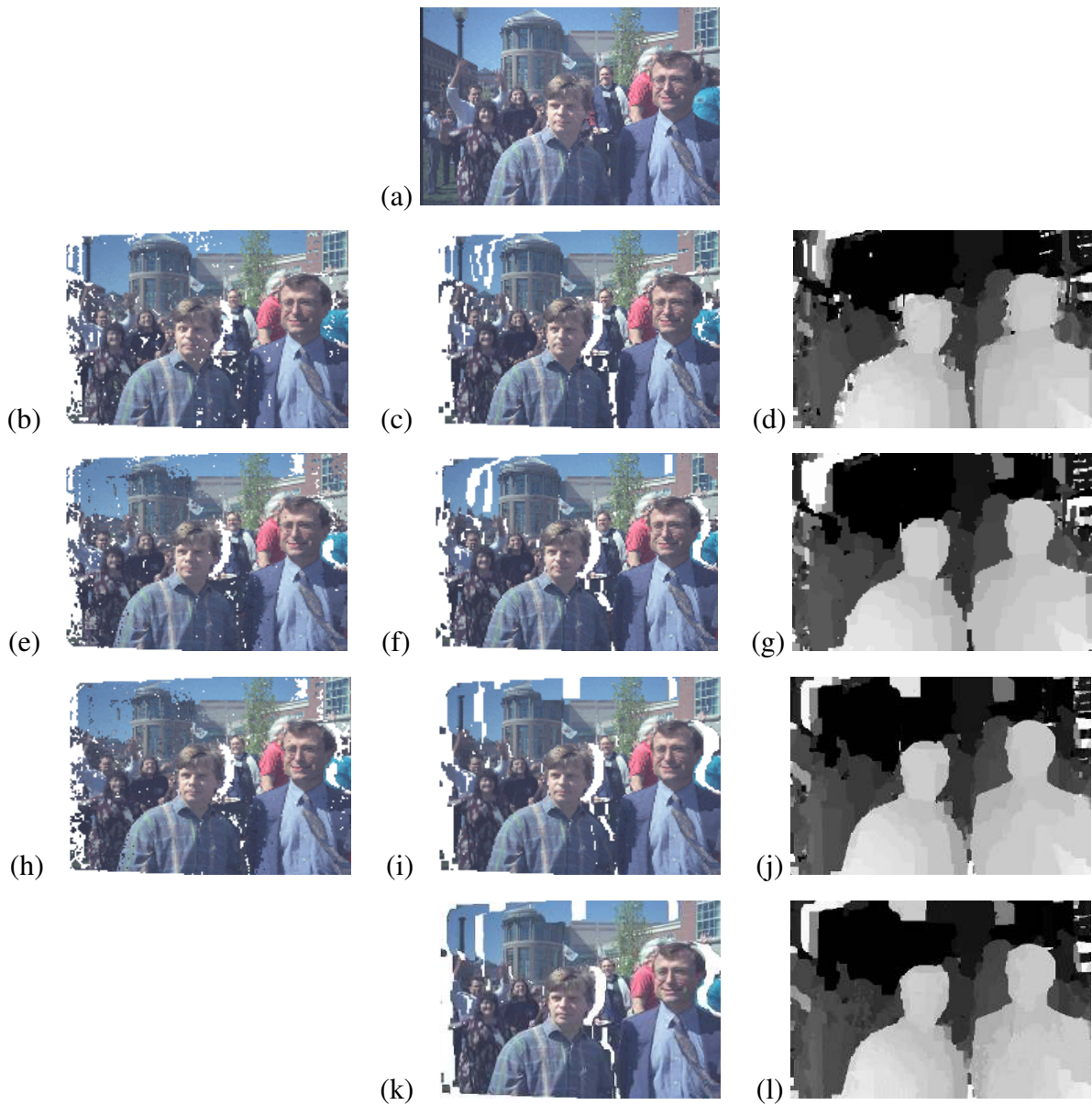
Figure 22: Examples of view reconstruction using results of graph cut (3x3 window used): (a) 1st frame of original 5-frame sequence (3rd frame is the reference), (b,c) Reconstructed view using all frames (before and after graph cut), (e,f) Reconstructed view using best frames (before and after graph cut), (h,i) Reconstructed view using best half sequence (before and after graph cut). (k) Reconstructed view after hierarchical graph cut. (d,g,j,l) are the respective depth maps after graph cut.
