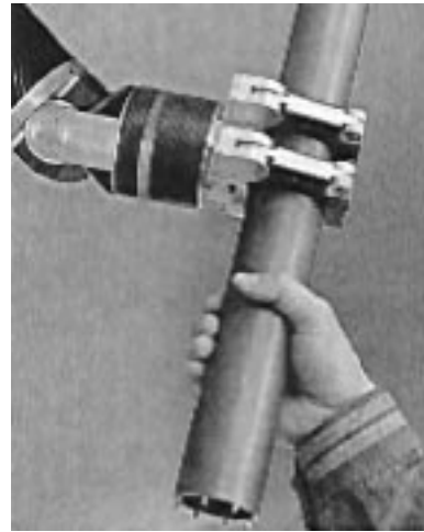
Fig. 2. Example of power grasping (courtesy of Barret Technologies, Inc.).
