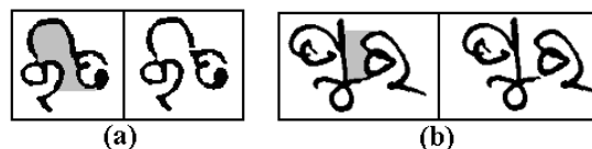
Fig.8. Examples of touching component segmentation using (a) biggest bottom reservoir (b) biggest top reservoir. Here reservoirs are marked by gray shades.
