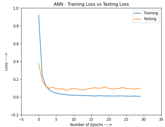
Figure 12. Graph illustrating the transition of training loss with increasing number of epochs in Multilayer Perceptron (Loss rate transition v/s number of epochs)
