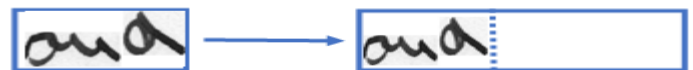
Fig. 4: Left: a picture from the dataset with an arbitrary size. it's scaled to suit the target image of size 128 \times 32 , the empty part of the target image is crammed with white color.
