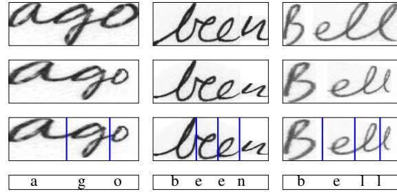
Figure 7. Examples of segmenting three distorted texts. (Top) Original texts. (Second row) Distorted texts. (Third row) Text segmentation using the proposed method. (Bottom) Character recognition from the class corresponding to the character likeliness.
