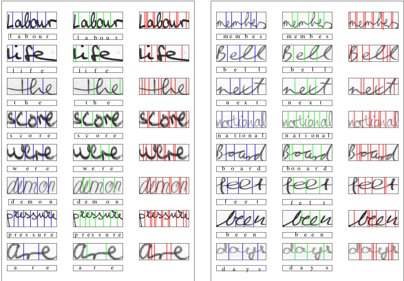
Figure 5. Text segmentation on a subset of the test words. For each test word, we show the segmentation from: (Left) the ground truth, (Middle) the proposed method, and (Right) the dynamic programming based method [17]. The characters below the test words for the proposed method (Middle column) are the recognition results from the character class corresponding to the character likeliness. The characters below the test words for ground truth (Left column) are the ground-truth characters for these words.
