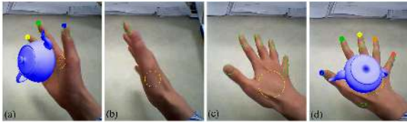
Figure 11. Flipping the hand from (a) to (d). (b) Fingertips are not detected because of self-occlusion. Then (c) fingertips are detected again when they are visible, (d) and rendering the object.
