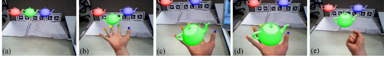
Figure 9. Selecting and inspecting augmented objects. (a) ARTag is used for stabilizing teapots in the world. (b) Selecting the green teapot in the middle, and then (c) inspecting it from (d) several angles. (e) As breaking fingertip tracking, the user releases the object.
