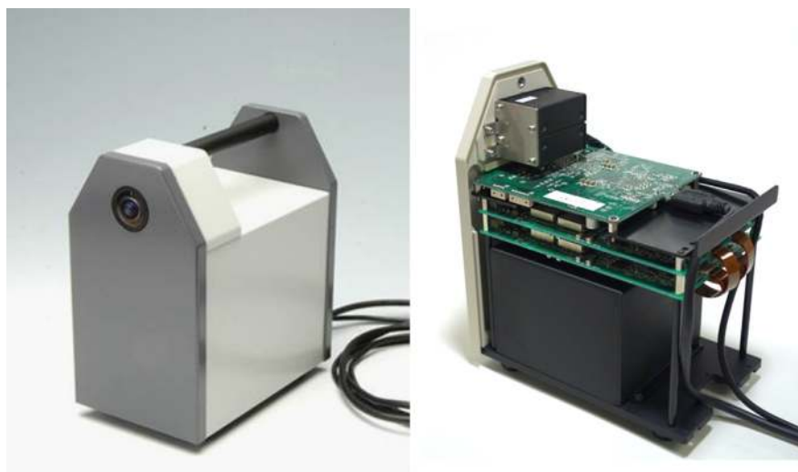
Fig. 6. Photos of the handy Compton camera prototype currently being fabricated by Hamamatsu Photonics K. K.
