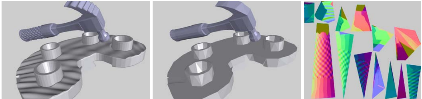
Figure 1: Haptic Display of Interaction between Textured Models. From left to right: (a) high-resolution textured hammer (433K polygons) and CAD part (658K polygons), (b) low-resolution models (518 & 720 polygons), (c) hammer texture with fine geometric detail.
