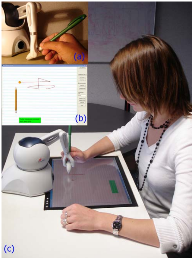
Figure 2. System overview: (a) The modified stylus pen; (b) The graphic User Interface displayed to the subject; (c) A subject undergoing training on the WYSIWYF interface. doi:10.1371/journal.pone.0001775.g002
