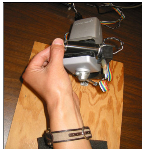
Figure 5 Participants held a haptically enabled knob through which haptic phonemes were displayed
