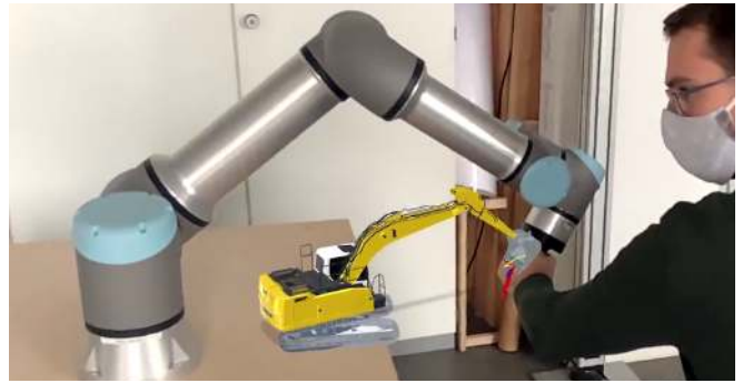
Fig. 8. Iviz visualization of the programming process for an excavator. The robot model is rendered in real-time onto the camera image of an Apple iPad.
