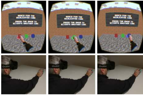
Figure 4. 1 for 3 Illusion - User touches 3 different virtual cubes while in reality the same cube is touched each time.
