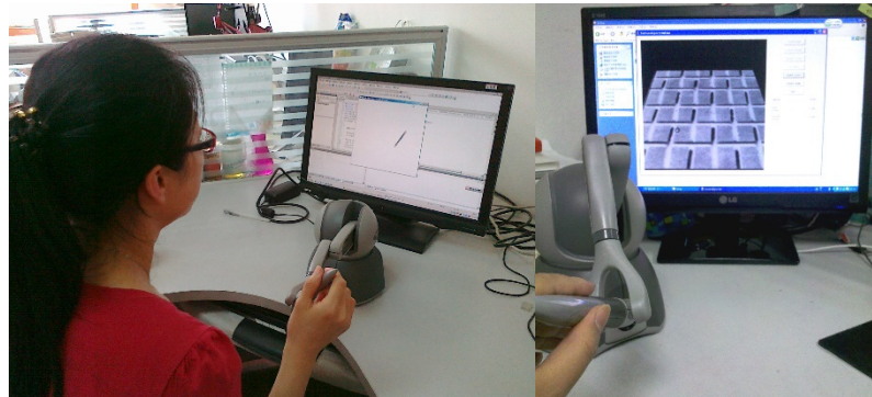
Figure 5. The experimental system of haptic texture rendering of 2D image.
