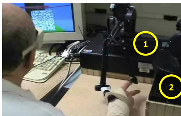
Fig. 1. Arrangement of two PHANToM devices. Two PHANToM devices were placed perpendicular to each other for the pinch movement
