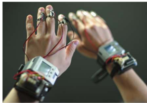
Fig. 3 Wearable finger vibrotactors can be used to encode Braille characters and for guidance and navigation for the blind. Image from [80] used with permission from IEEE
