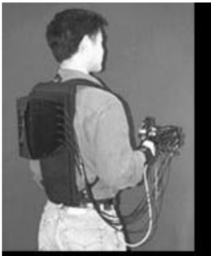
Figure 11. The GraspPack™ extension to the CyberGrasp haptic glove [22]. Reprinted by permission
