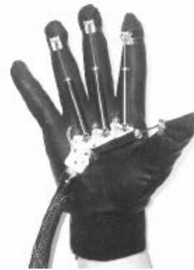
Figure 12. The Rutgers Master II-New Design haptic glove [17].
