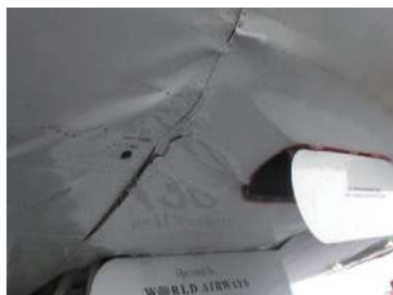
Fig. 2. DC-10 hard-landing accident at Baltimore/Washington International Thurgood Marshall Airport on May 6, 2009. [4]
