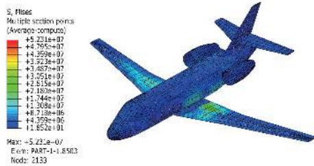
Fig. 30. Result of linear dynamic analysis with EIR method at 0.25s
