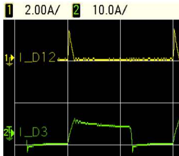
Figure 2.8: Experimental results of the two-switch flyback converter at V_I = 60 V and P_O = 30 W. Top trace: clamping diode current waveforms i_{D1}, i_{D2} (2 A/div.); Bottom trace: rectifier diode current waveform i_{D3} (10 A/div.). Horizontal scale: 5 \mu\text{s}/\text{div} .
