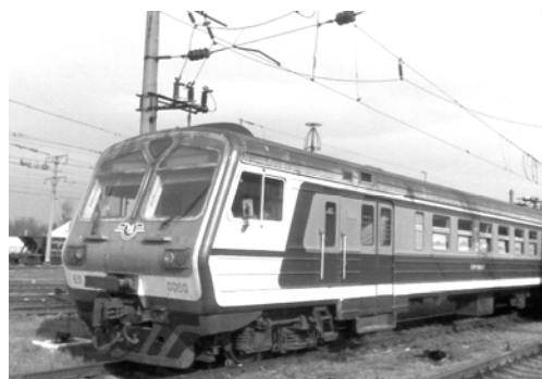
Fig. 1. The head car of the electric train ED9M
