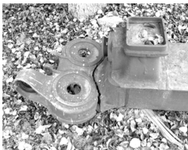
Fig. 5. General view of the fractured beam
