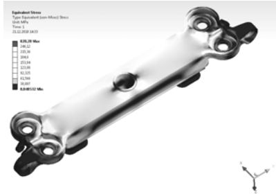
Fig. 12. Stress distribution field during motion of electric train in traction mode with small strengthening rib
