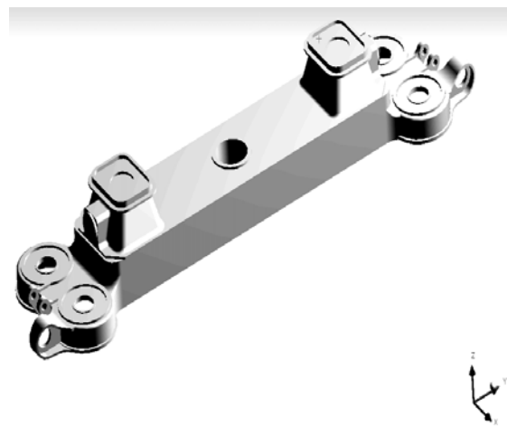
Fig. 6. General view of the model of central suspension beam for the electric train ED9M
