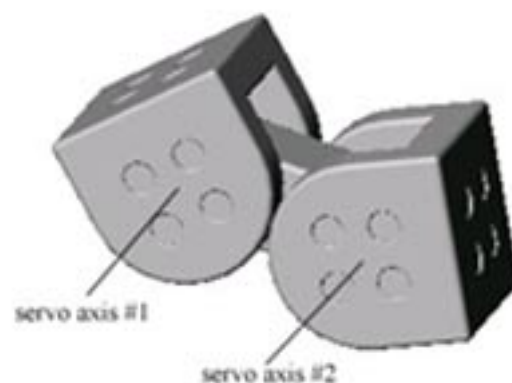
Figure1 CAD model of robotic module In the following sections, we describe features of this module.
