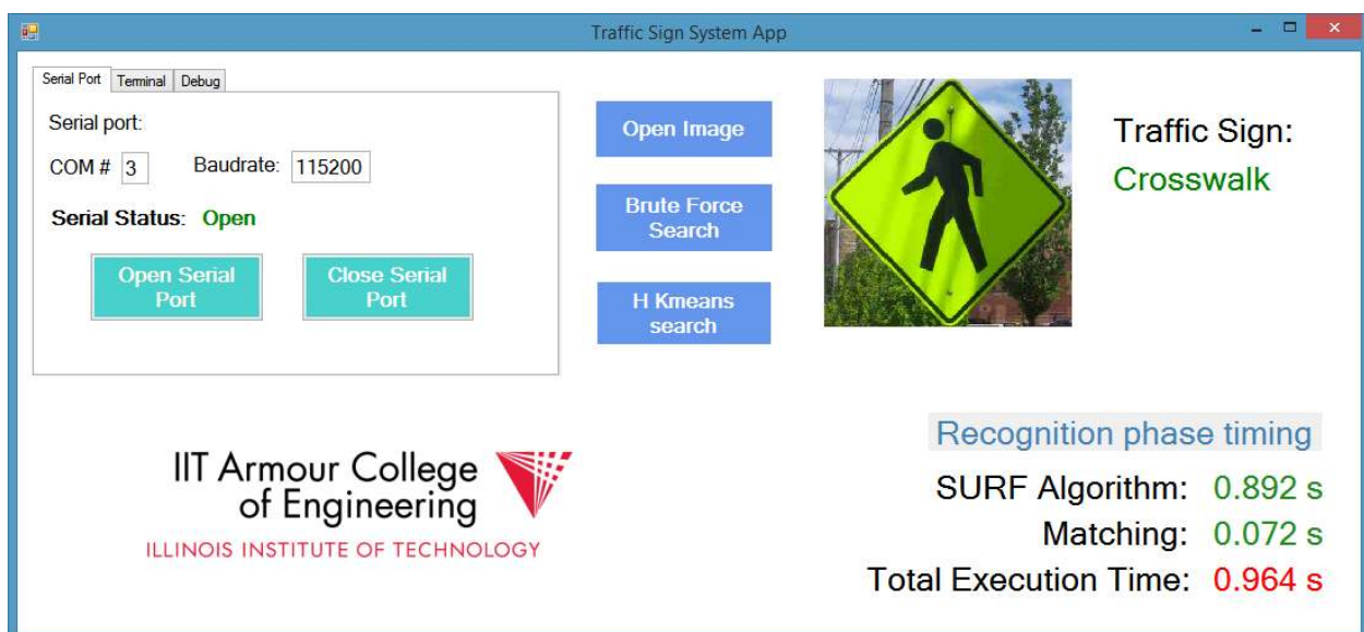
Figure 23. Execution time for the (recognition phase only) “CROSSWALK” sign using k -means matching.
