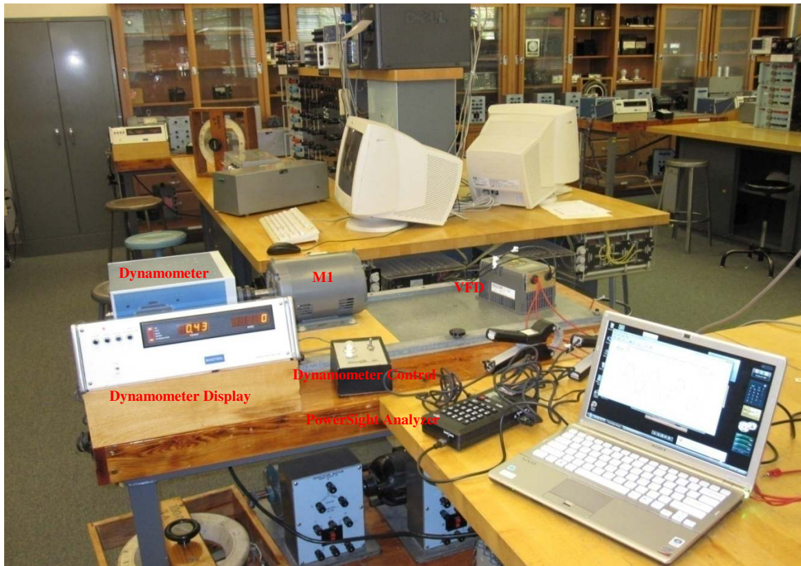
Figure 4.7 - Motor 1 and VFD Picture
