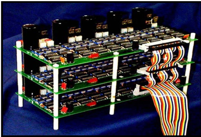
Fig. 8. 10 kW multilevel converter prototype
