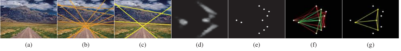
Figure 5: Illustration of the proposed algorithm: (a) input image, (b) selected lines through the selection-and-removal process, (c) semantic lines, (d) probabilities of line candidates in the Hough space, (e) node set corresponding to the selected lines, (f) complete graph, (g) maximal clique. In (f), an edge is depicted in green or red depending on whether its weight is above the threshold \kappa in (8) or not. As the weight approaches zero, the transparency increases.
