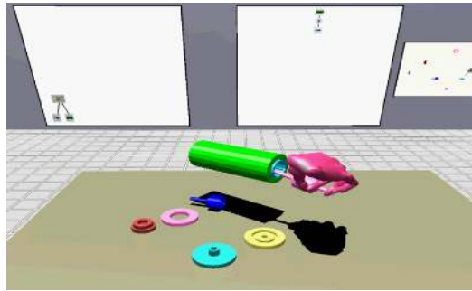
Fig. 11. Assemblability testing and generation of assembly plans in VE [23]
