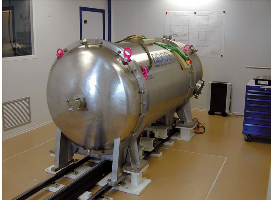
Figure 2: The closed HARPS vacuum vessel in the Geneva integration laboratory.
