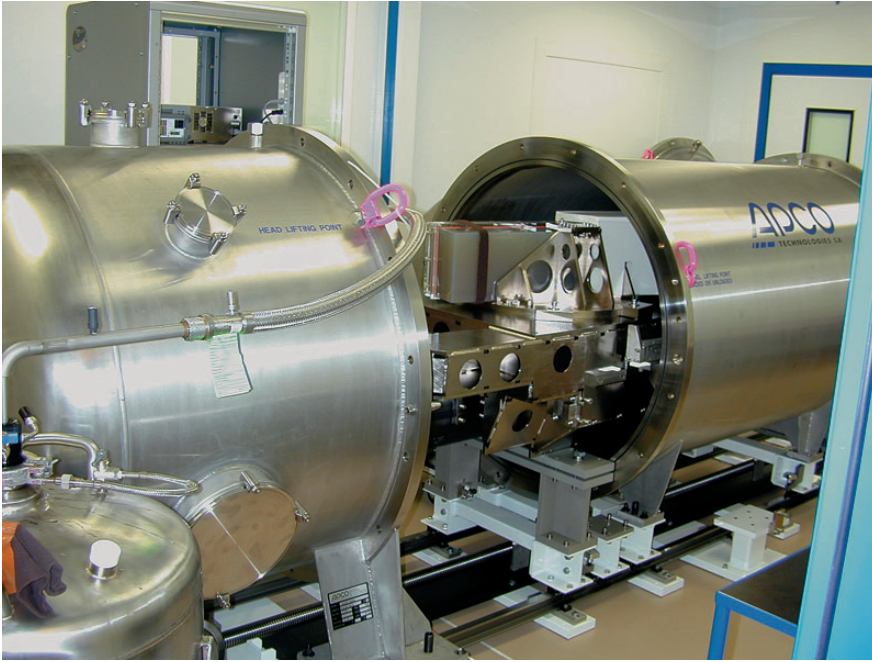
Figure 3: The open HARPS vacuum vessel. The back side of the echelle grating is visible on top of the optical bench as well as the rail system used for moving the large parts of the vessel.
