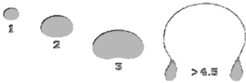
Fig. 3 Change of shape of raindrop with the diameter
