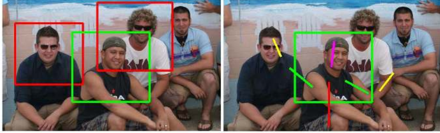
Fig. 4. Overlap features. Left: Three overlapping detection windows. Right: the HPE output is incorrect due to interference from the neighbouring people. This problem can be flagged by the detection window overlap (output from Eichner and Ferrari [5]).
