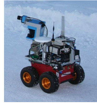
Fig. 5. Our mobile robot platform “Tjorven” equipped with the sensors used in this paper: the SICK LMS 200 laser range scanner and a colour CCD camera both mounted on an Amtec pan tilt unit.
