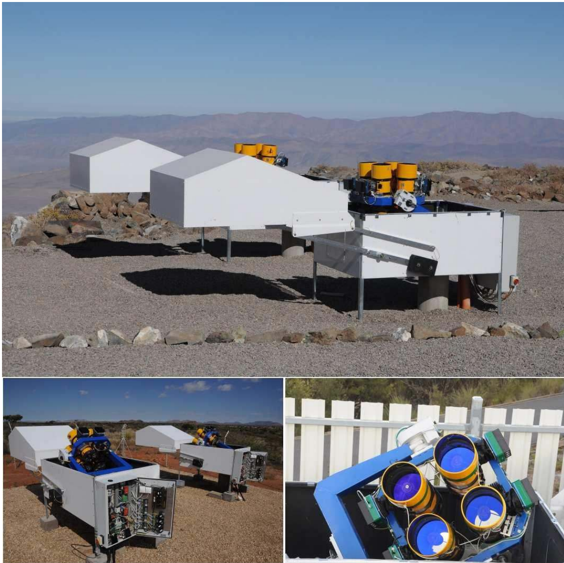
FIG. 5.— The HS 4 units at Las Campanas Observatory, Chile (top), with the telescopes pointing towards the zenith. The HS 4 units at the HESS site in Namibia (bottom left), with telescopes stowed towards the south celestial pole. The electronic boxes are open showing the dome and telescope electronics described in § 2.1.5. A close-up view of an HS 4 unit at Siding Spring Observatory in Australia (bottom right), with part of the wind fence visible in the background.
