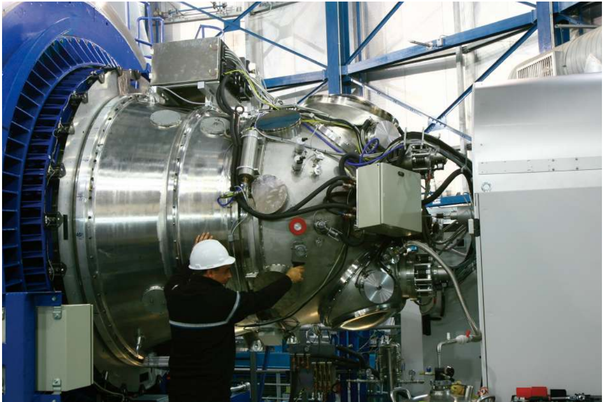
Fig. 1. HAWK-I on the telescope, attached to the Nasmyth focus of the Unit Telescope 4 of the ESO VLT. On the left in blue: the adapter/rotator of the telescope. On the right in light grey: the cable co-rotator fixed on the Nasmyth platform.
