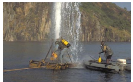
In one night, 1,700 people and many livestock were suffocated by CO 2 from Lake Nyos. A 1995 expedition has since tested degassing equipment.
