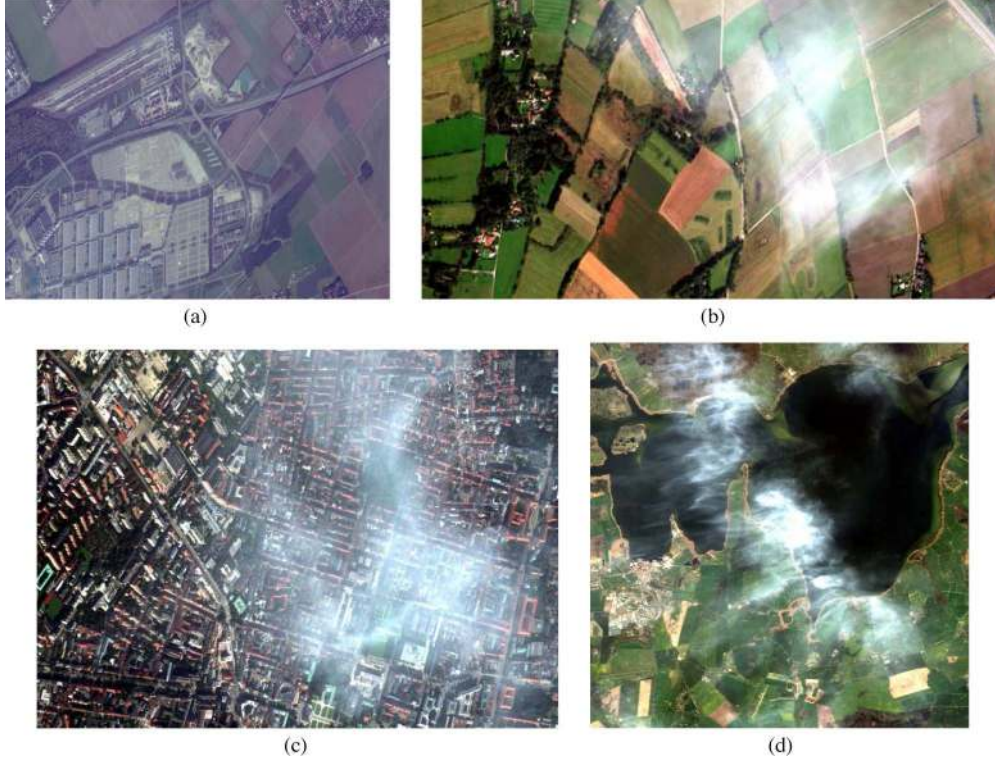
Fig. 1. Typical types of haziness in optical imagery. (a) Uniform haze (WorldView-2). (b) Moderately thick haze (WorldView-2). (c) Moderately thin haze (WorldView-2). (d) Thick structured haze (AVNIR).
