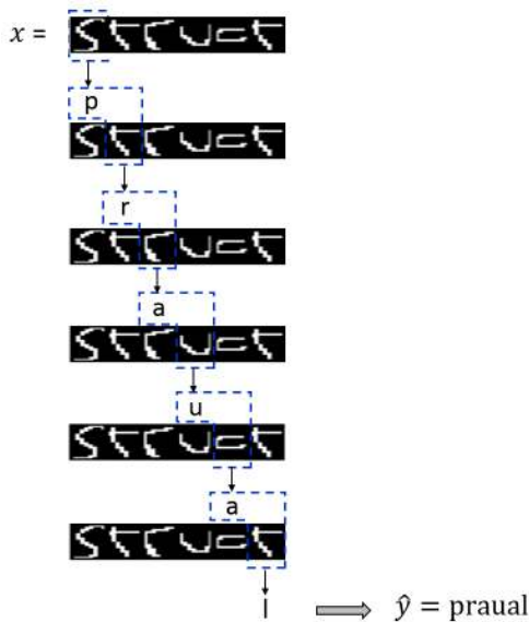
Figure 6: Illustration of recurrent classifier for handwriting recognition problem. The classifier predicts the labels in a left-to-right order. It makes the labeling decision at each position greedily based on the character image and the predicted label at previous position (shown by the dotted box). In this particular example, the classifier makes a mistake at the first position and this error propagates to other positions leading to a very bad output.
