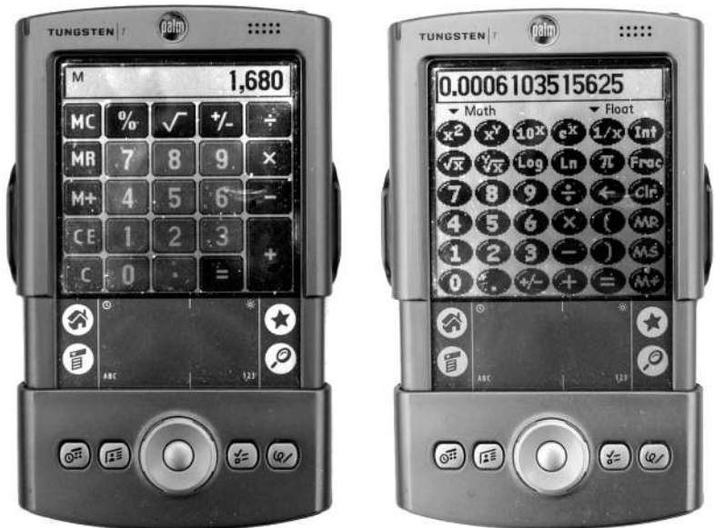
Figure 2. With soft buttons, the same display surface can easily be used for different button layouts and functionality—all defined by software. This example shows two different calculator applications on a Palm Pilot. To the left, a simple standard calculator; to the right, a scientific calculator.
