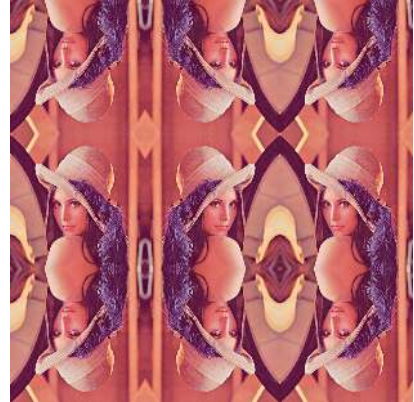
Fig. 1: The example of expanding an image by mirroring in vertical, horizontal and diagonal direction.
