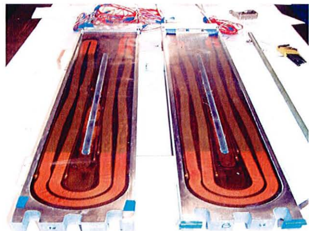
Figure 3: Modules A & B, fully impregnated and with voltage tap/quench heater traces.
