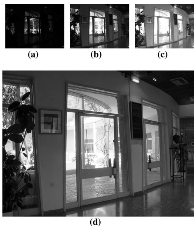
Fig. 1 HDR frame of a real scene captured with three different exposure times (sequences by Fattal et al. [14]). a Low exposure, b middle exposure, c high exposure, d HDR image
