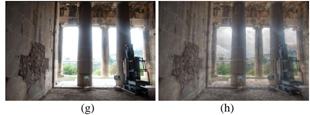
Figure 2: Scene 2, (a) – (g) 7 frames with exposure values from -3EV to +3EV (h) tone mapped image according to Mantiuk's algorithm (Mantiuk et al., 2006).
