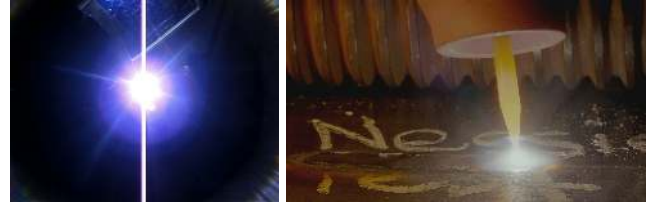
Figure 2: (Left) State-of-the-art digital cameras can not capture extreme dynamic range of TIG welding. The electric arc is overexposed, yet the surroundings are underexposed. (Right) Single frame from the real-time HDR video glasses. Our system captures 120 frames/sec.
