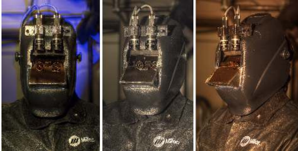
Figure 1: EyeTap welding helmet causes the eyes themselves, to, in effect, become both cameras and displays by providing exact POE (Point-of-Eye) capture for a stereo headup display.
