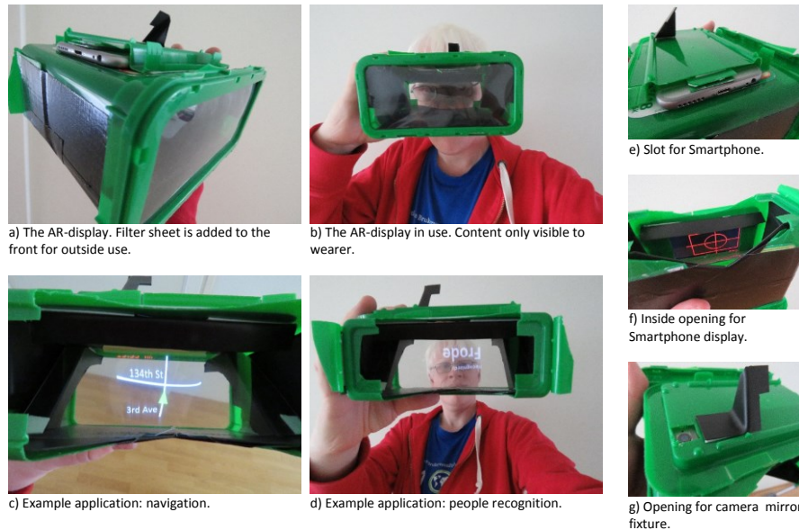
Fig. 4. The homemade wearable augmented reality Display. a) the overall device, b) the augmented information is not visible to onlookers, c) and d) augmented information as seen by the user, d) and e) the augmented image from the smartphone and f) camera-mirror fixture.
