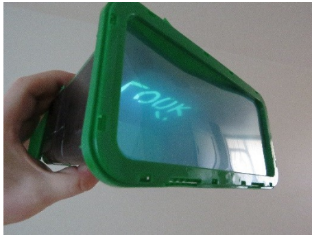
a) Headset with a 4-layer green filter.
