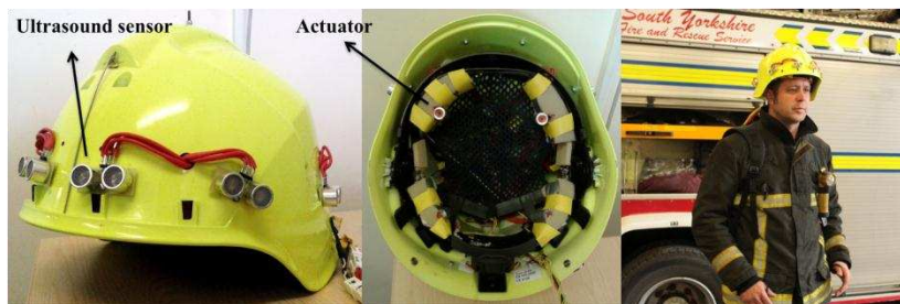
Fig. 1. The first generation ‘Tactile Helmet’ [6] was composed of a ring of ultrasound sensors and four actuators inside the helmet and was designed to help firefighter’s navigate inside smoked-filled buildings.
