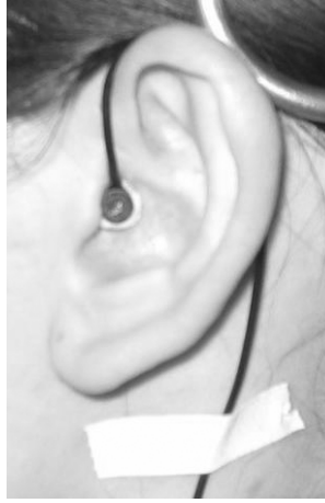
Figure 3. Blocked-ear-canal measurement with miniature microphone
