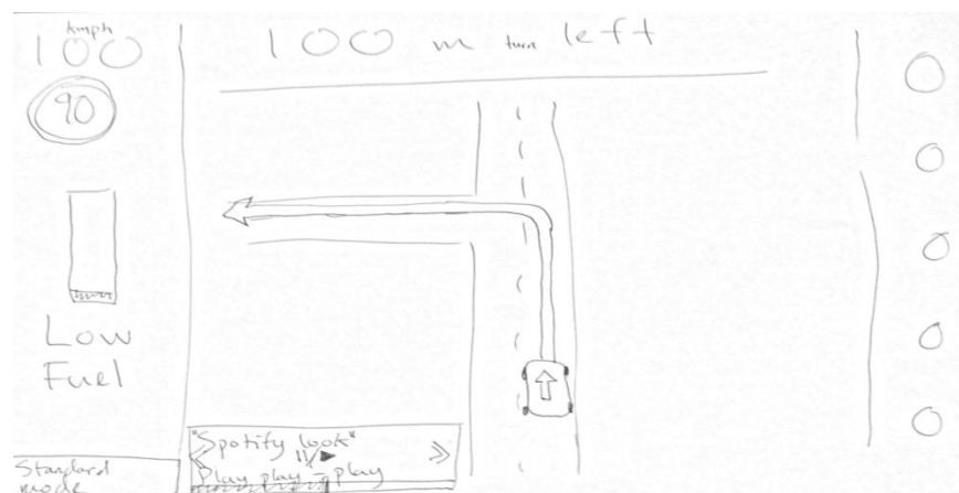
Figure 16. Early sketch of HUD design and layout
