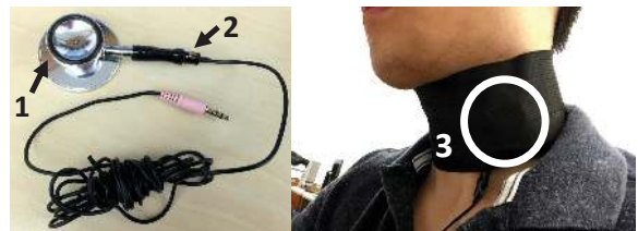
Fig. 8: The hardware for audio-based sensing. (1) A chestpiece of a clinical Elite 4000 stethoscope. (2) A unidirectional condenser microphone. (3) The chestpiece attached to skin using an elastic band.
